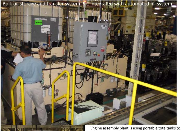
deliver engine oil to automated fill stations on the assembly line. Two engine oils are being dispensed. The systems include secondary lower tanks and containments to provide continuous operation – no shut down when the tote runs empty.
